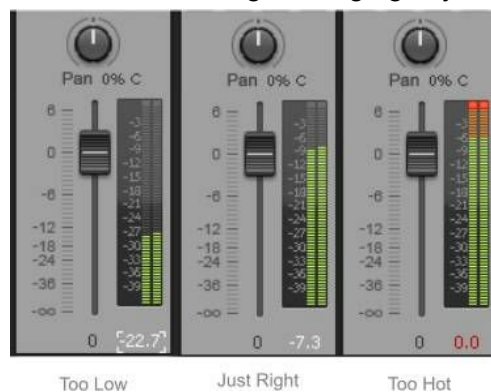
Set proper levels to leave plenty of headroom and avoid clipping: gain staging
